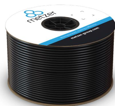
Micro Tubes play a critical role in micro irrigation systems, especially in orchards, greenhouses, and nurseries. They are widely used with micro sprinklers, drippers, and automation systems to provide precise irrigation solutions. Manufactured using PVC or Low or Medium density polyethylene, their durability and ability to operate under various climatic conditions and water pressure up to 6 bar make them suitable for various agricultural needs.
